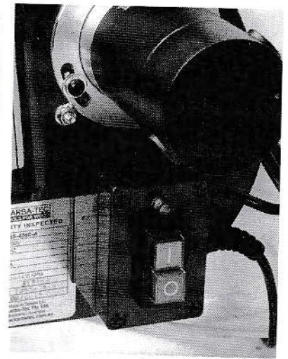
NVR power isolating switch
